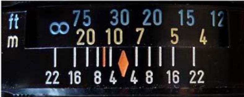
This image shows an older lens focused at about 30 feet. The depth of field scale shows the range of distances that would be in acceptable focus for various aperture settings.
