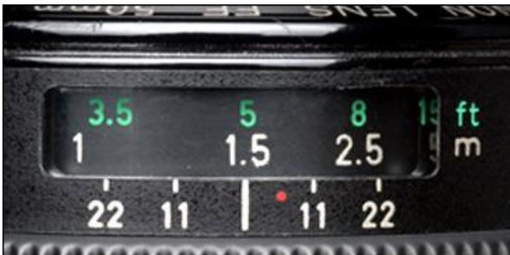
This lens is focused at 5 feet. The depth of field scale shows:
