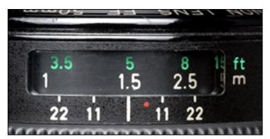
This lens is focused at 5 feet. The depth of field scale shows:
