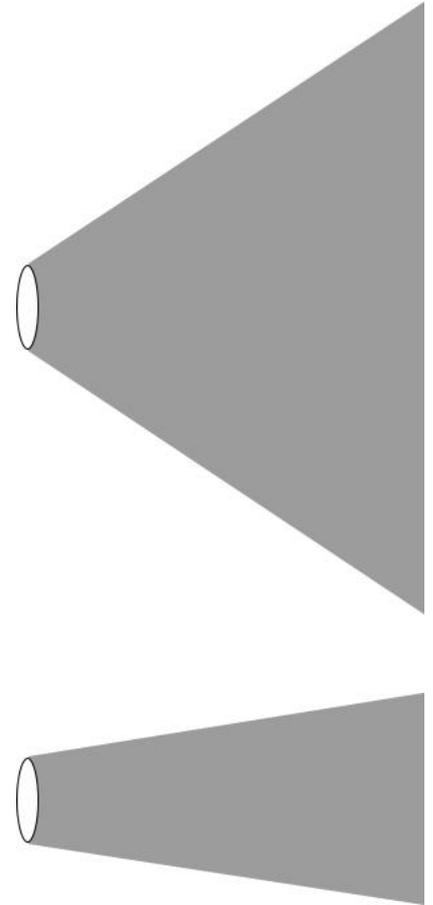
Instead, we measure the size of the opening in the lens as a ratio of its diameter to the focal length of the lens.
